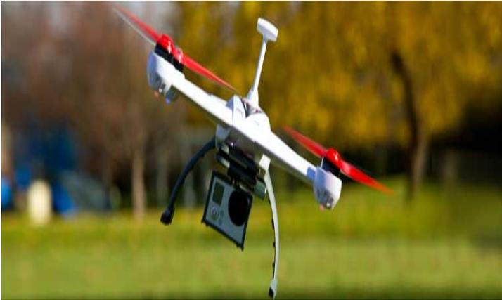
What makes the Blade 350 QX3 such a great camera platform? Safe (Sensor Assisted Flight Envelope) technology. Using this technology, the Blade 350 QX3 gives you two flight modes have been specialty programmed for aerial videos and images. Both features self-leveling and use GPS and altitude sensor precisely hold position in hover. Safe Technology will even land the aircraft for you if you activate the return home function.
